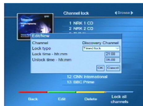
**Figure 33 – locking a specific channel**
